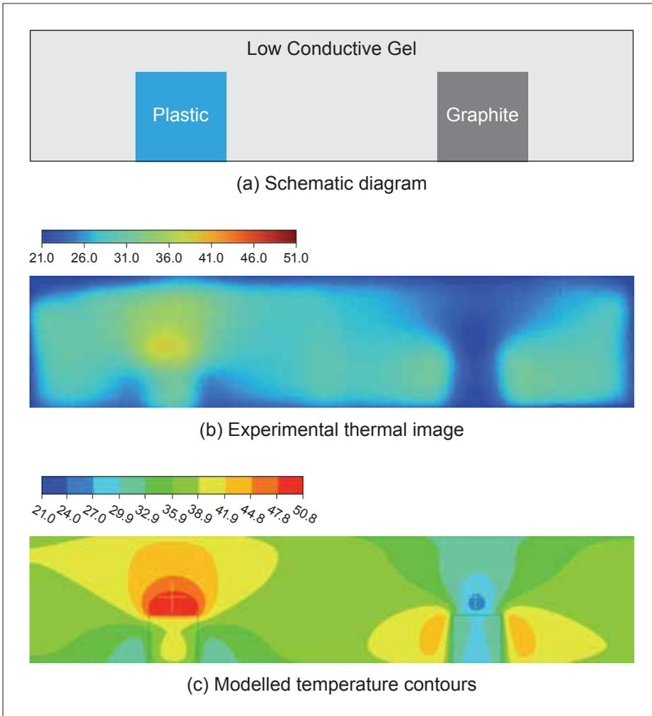
Figure 1. The simplified heterogeneous structure made from low conductive gel, with submerged plastic and graphite blocks.
